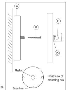
· Seal the screw fixings to maintain the IP rating of the fitting.
