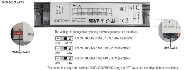
Choose your preferred wattage and colour before installing by wattage switch or CCT switch on the driver. Note: Befeore you change the wattage or colour, please turn off the power switch for safety.
