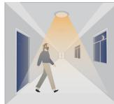
With insufficient daylight, the sensor turns light ON when motion gets
