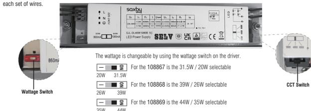
The colour is changeable between 3000/4000/6000K using the CCT switch on the driver before installation. Choose your preferred wattage and colour before installing by wattage switch or CCT switch on the driver. Note: Befeore you change the wattage or colour, please turn off the power switch for safety.
