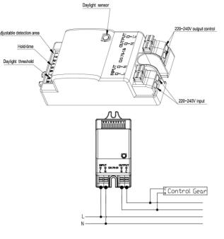
\*50%, 75%, 100% detection sensitivity is workable when installed at 6m mounting height. Only 10%, 25% sensitivity is not able to detect motion signal.
