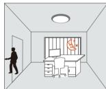
With movement and insufficient If there is no more movement, dimming level after hold-time.
