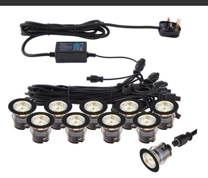
An addition to the popular IkonPRO recessed LED decking kit range, within each head there is the choice of 3000K or 4000K. Using the unique design of removable and interchangeable heads to change colour, you simply lift the LED head out of the connector, turn the head 180° and reinsert into the loom. Designed to be fitted and wired during the decking build stage without the heads, the supplied rubber caps protect the fitting from the elements until the decking is complete.
